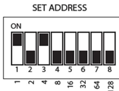
Each sensor must have a unique address on the network. The address is set by means of a DIP switch (SW100).
