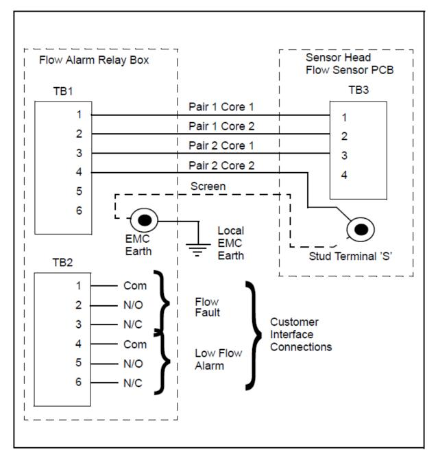
Figure 26. Flow alarm interconnection wiring schematic
