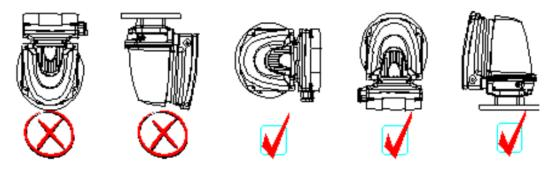
Figure 2 - Sensor Head mounting orientation
