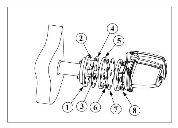
Figure 8. Probe retention flange installation
