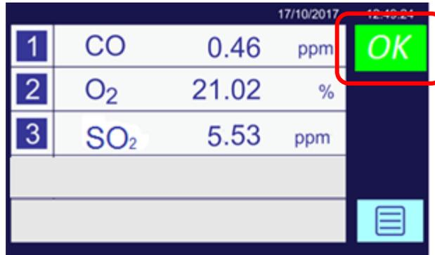
Figure 4-7: Home screen (three gas transducers)
