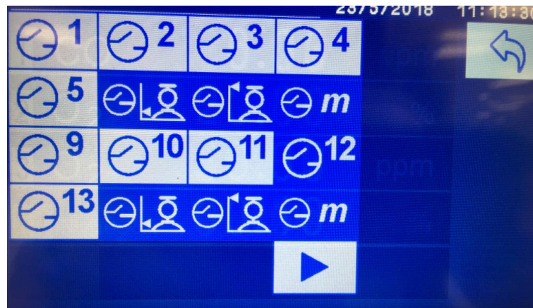
Figure 10-11: Available relays on the system with Auto-Cal pre-assigned relays.
