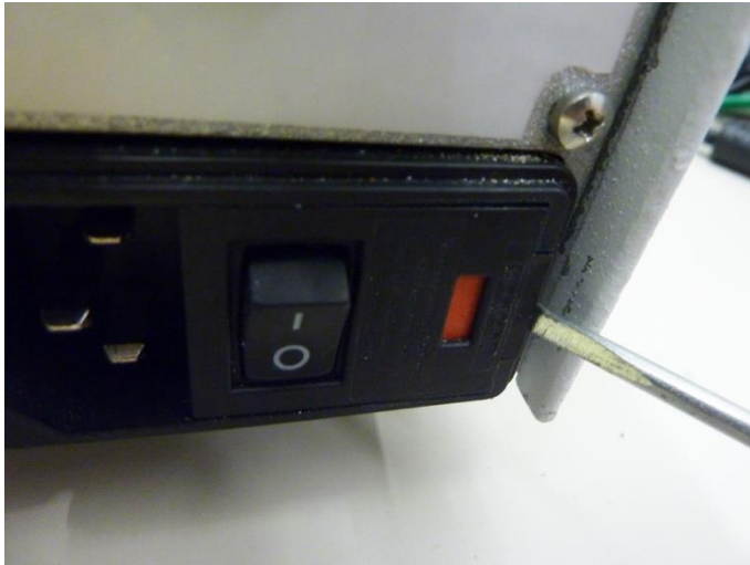
Figure 13-1: Open the fuse panel
