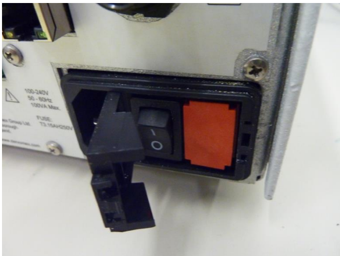
Figure 13-2: Fuse panel opened
