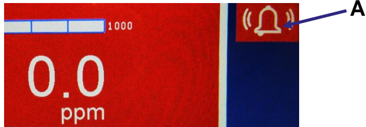
Figure 7-13: Measurement alarm condition triggered
