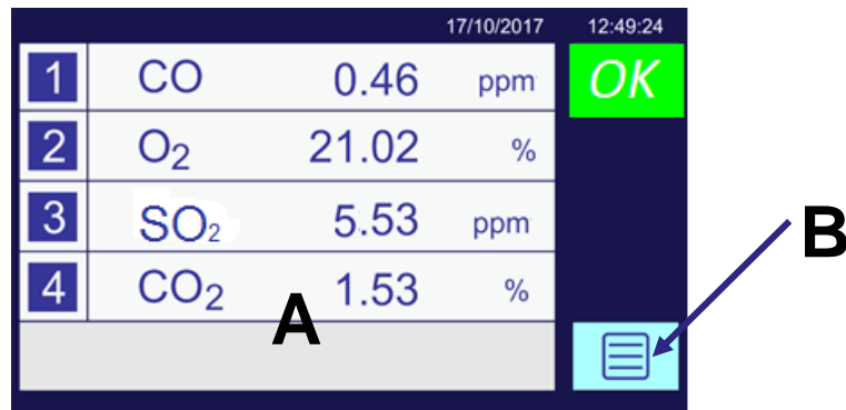
Figure 5-2: Home screen for a 4-transducer analyzer (A) is the Main Selection Touch Screen and (B) indicates the Main Menu Icon
