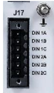
Figure 11-21. Jumper 17 used for Auto-Cal configurations.
