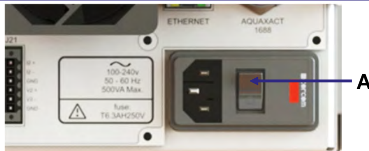
Figure 4-6: On/off switch on the rear of the analyzer
