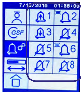
Figure 5-35: Alarm icons on alarm screen
