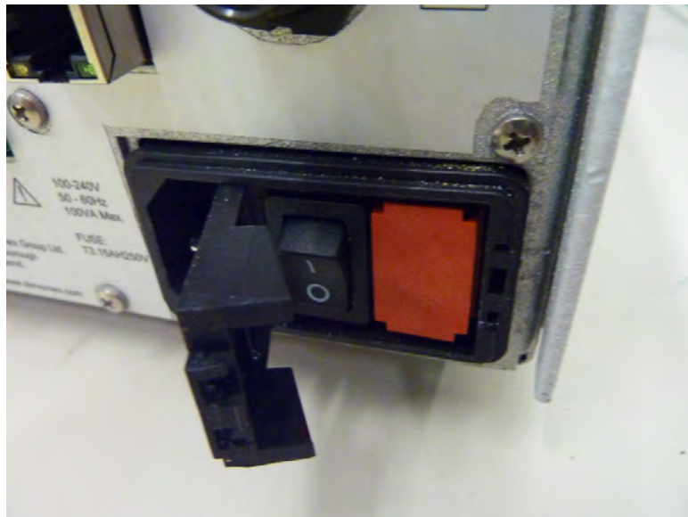
Figure 8-2: Fuse panel opened
