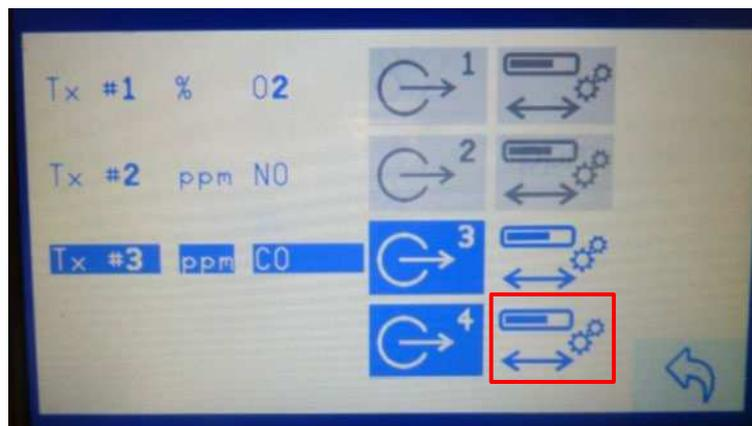
Figure 10-37: Second Analog Output assigned to transducer
