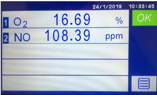
Figure 7-24: NO measurement displayed on Main Screen
