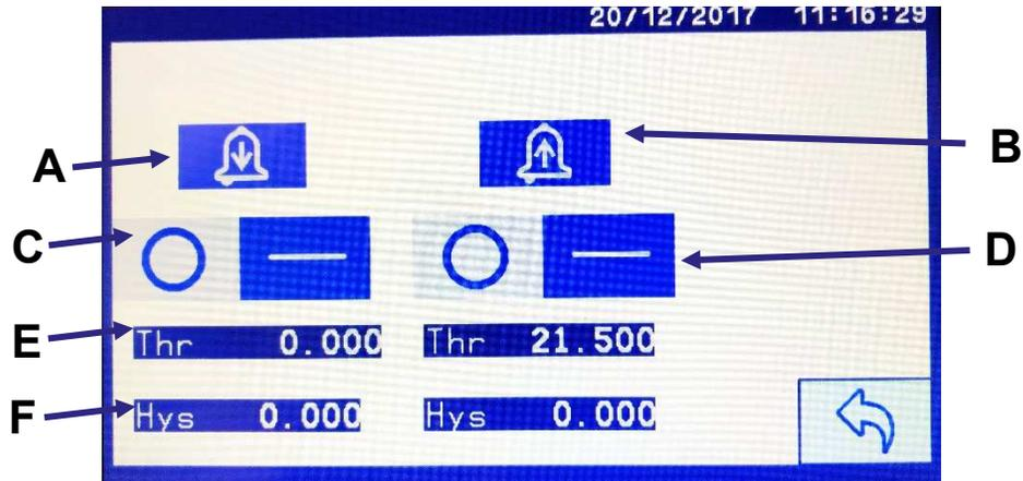
Figure 10-23: Settings Communications-Analog Input Alarm setting screen
