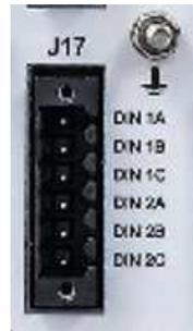
**Figure 11-21. Jumper 17 used for Auto-Cal configurations.**
