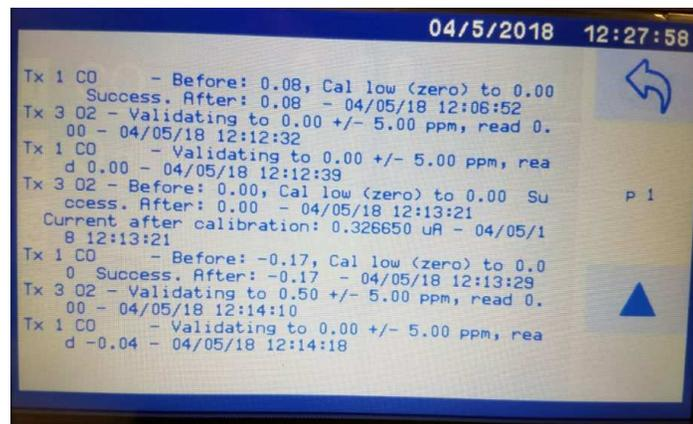
Figure 11-23: Cal log file displayed on screen
