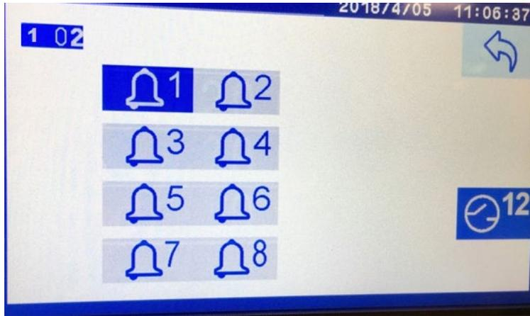
Figure 10-13: Alarm assignment screen for O<sub>2</sub> (Relay #12)
