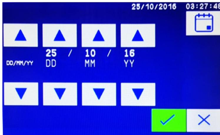
**Figure 10-18: Set the analyzer date screen**
