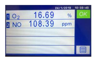
Figure 7-24: NO measurement displayed on Main Screen
