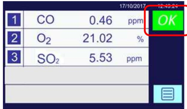
**Figure 5-6: Home screen (three gas transducers)**
