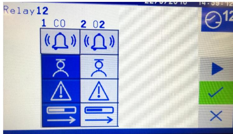
**Figure 10-12: Activity Assignment Menu for Relay #12 in an analyzer with two transducers (CO and O<sub>2</sub>).**
