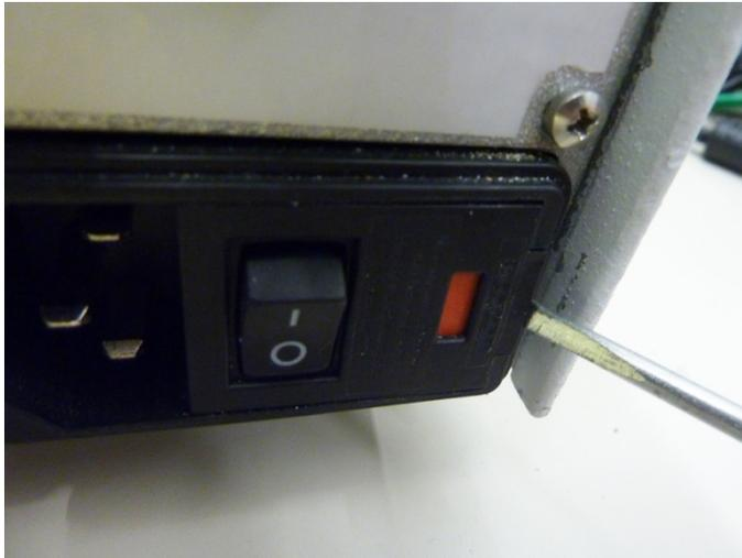
**Figure 13-1: Open the fuse panel**
