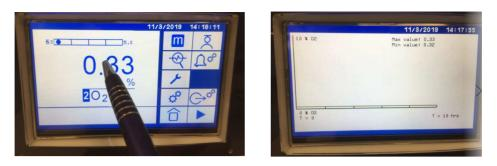
Figure 7-22: Showing data recording plot – Touch center of screen (left) and Data Recording Plot screen (right)
