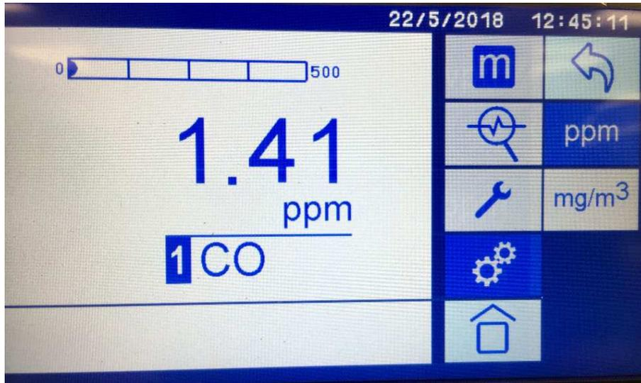
Figure 10-26: Data Units screen showing ppm selected units (mg/m<sup>3</sup> is not selected).
