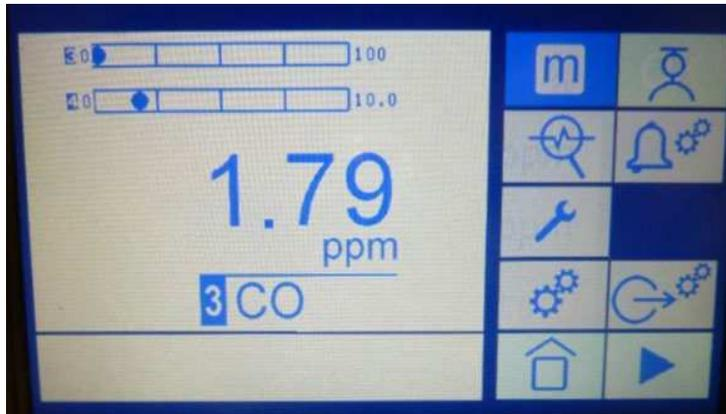
Figure 10-38: Measurement screen showing two analog outputs
