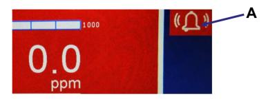
Figure 7-13: Measurement alarm condition triggered
