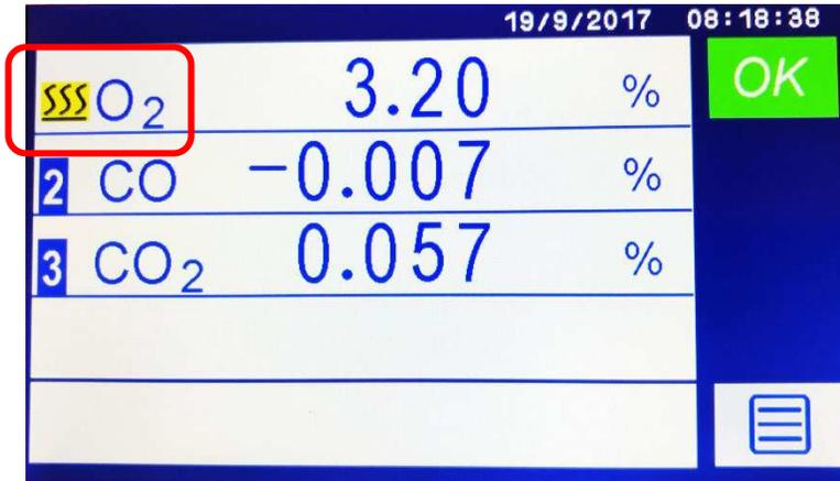
Figure 4-3: Home screen for a 3-transducer analyzer showing the O<sub>2</sub> warming up
