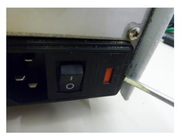
Figure 13-1: Open the fuse panel
