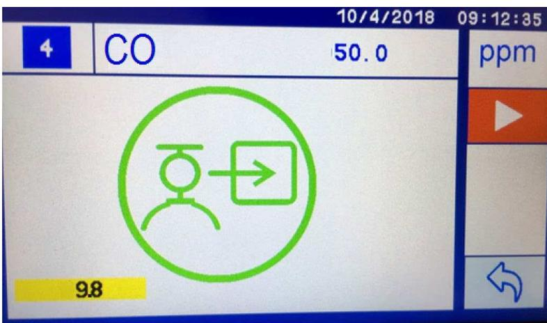
**Figure 11-3: Start calibration – gas filling state**
