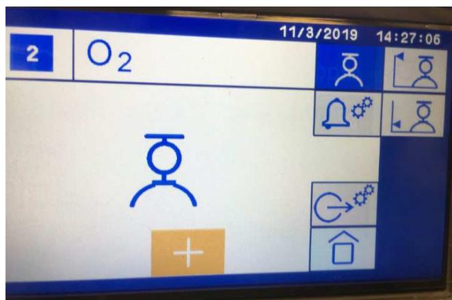
**Figure 10-31: Add Assignment mode activated, manual calibration section**
