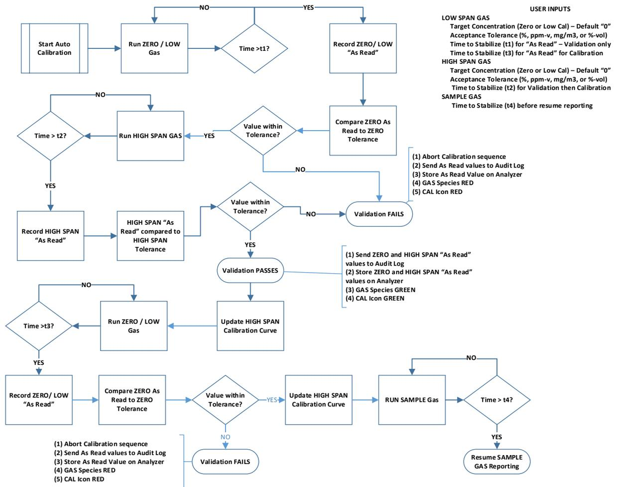
Figure 11-12: Flow diagram of the Auto-Calibration Steps
