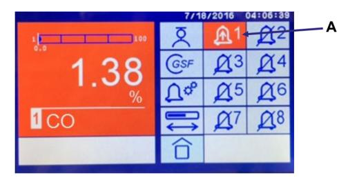
Figure 7-14: Alarms screen showing Alarm #1 (A) High Measurement Range triggered
