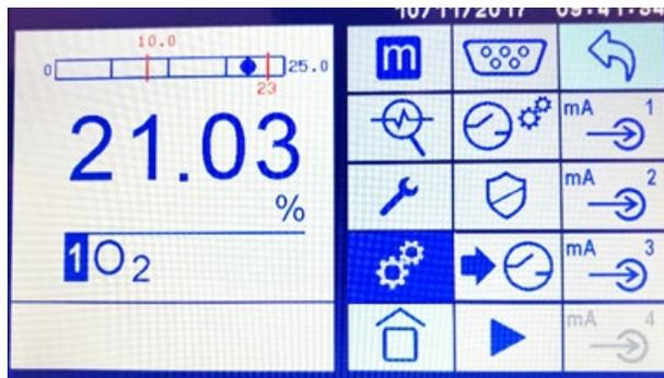
Figure 10-21: Active mA Analog Inputs that are purchased appear as blue pictures / text
