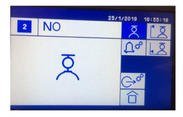
Figure 11-1: Calibration screen (manual calibration activated)
