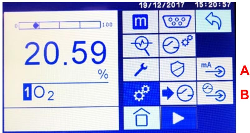
Figure 10-20: Settings sub-screen for mA Analog (A) and Digital (B) Inputs
