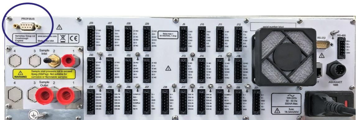
Figure 17-1: PROFIBUS connection on rear of the analyzer
