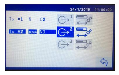
Figure 7-16: Select measurement (Tx #) for range setting
