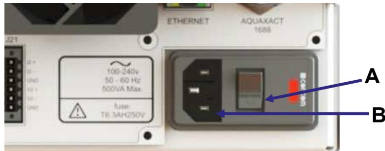
**Figure 3-5: Power switch (A) and electrical supply socket (B) on rear of analyzer**
