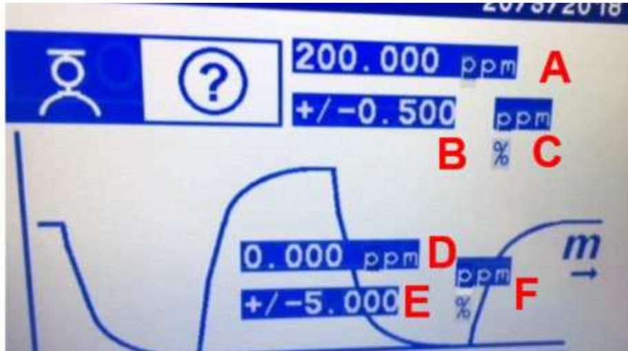
Figure 11-16: Auto-Cal thresholds setup (auto-calibration is active)
