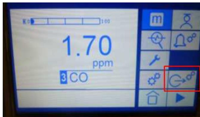
**Figure 10-35: Measurement page – Analog Output Settings icon**
