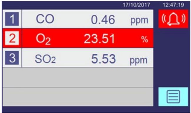
Figure 5-7: Home screen (3 transducer analyzer), showing O<sub>2</sub> alarm
