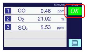
Figure 5-6: Home screen (three gas transducers)
