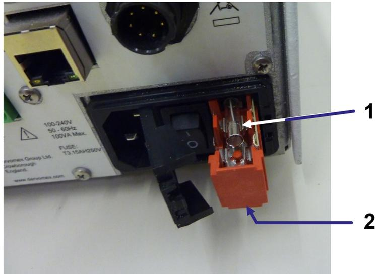
**Figure 13-3: Pull out the red fuse holder**
