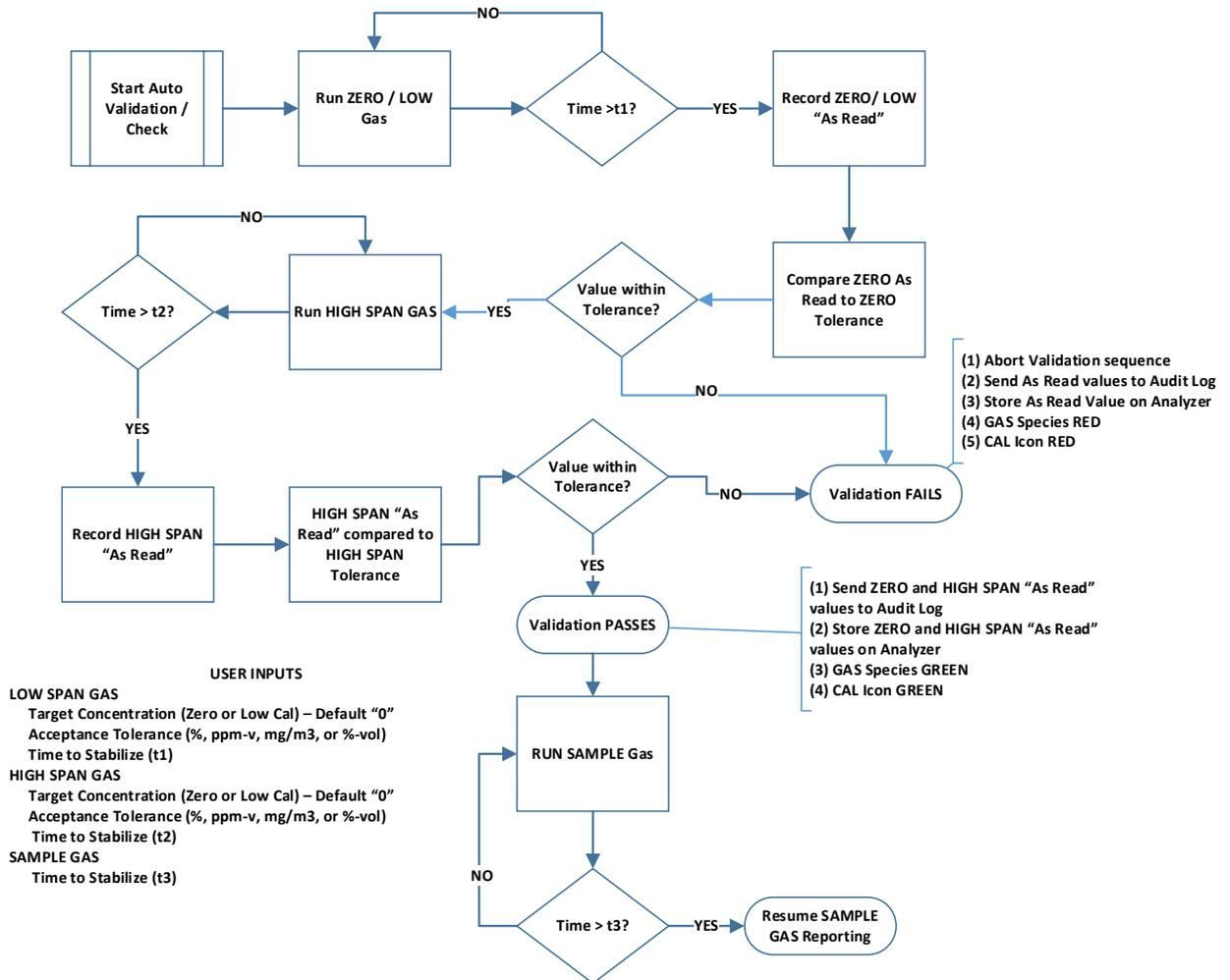
Figure 11-8: Flow diagram of the Auto-Validation steps
