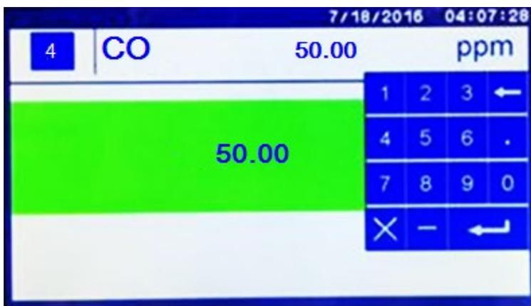
**Figure 11-2: Span value entry keypad with Target Value on the top bar**
