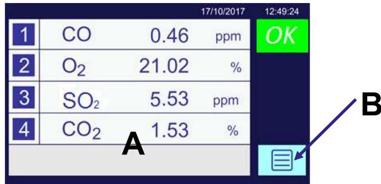
Figure 5-2: Home screen for a 4-transducer analyzer (A) is the Main Selection Touch Screen and (B) indicates the Main Menu Icon
