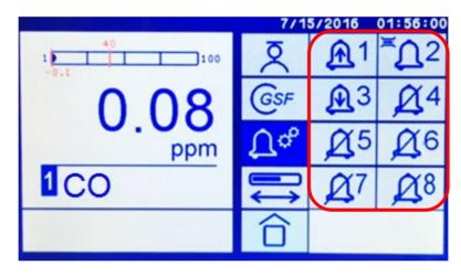
Figure 7-6: Alarms screen showing CO with 8 alarms available: #1, #2, #3 have already been configured.
