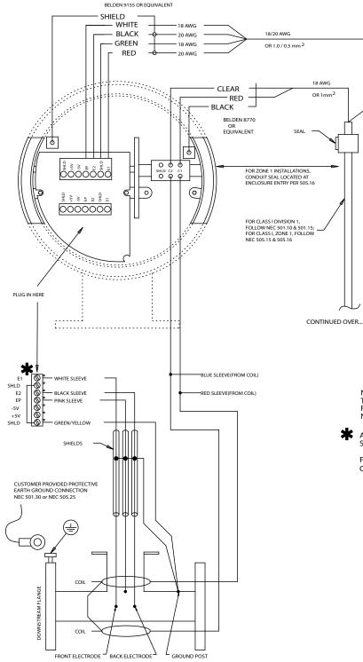
NOTE: THE TOTAL RESISTANCE OF THE GROUND CONNECTION FROM THE DETECTOR TO THE AMPLIFIER CAN NOT EXCEED 1 OHM
