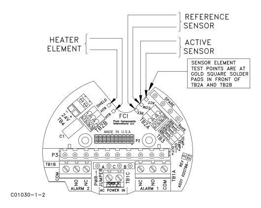
Figure 23 – Terminal Board, Test Points
