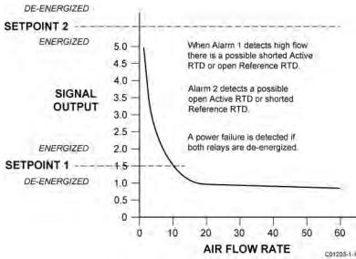
Figure 20 – High Flow Fail-Safe Alarm
