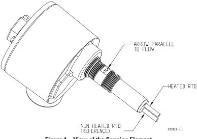
Figure 1 – View of the Sensing Element
