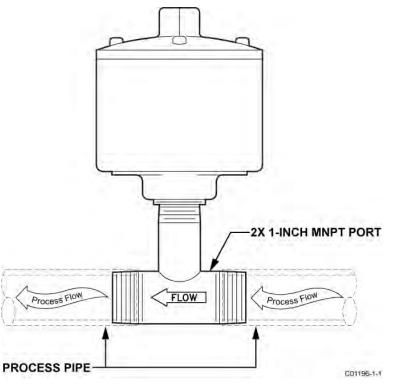
Figure 4 – FLT93L In-Line Flow Element (Shown with 1-Inch MNPT Ports)
