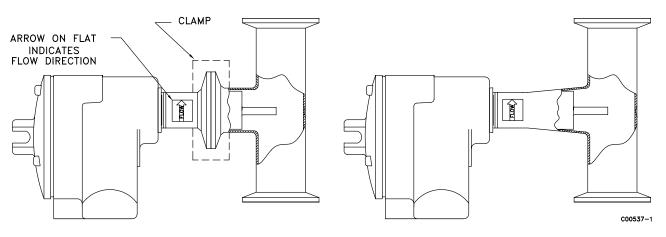
Figure 5 – FLT93C Sanitary Flow Elements (RC and CIP)
