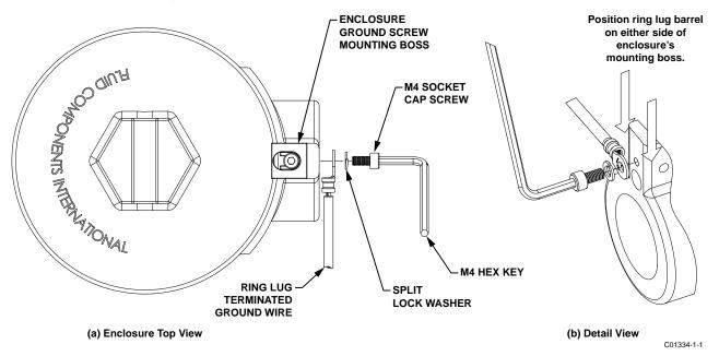
Figure 8 – Installing Ring Lug Terminated Ground Wire
