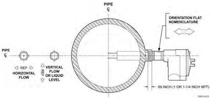
Figure 2 – NPT Pipe Thread Mount
