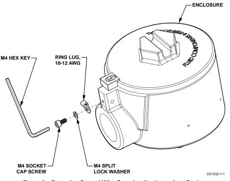
Figure 6 – Removing Ground Wire Securing Hardware from Enclosure
