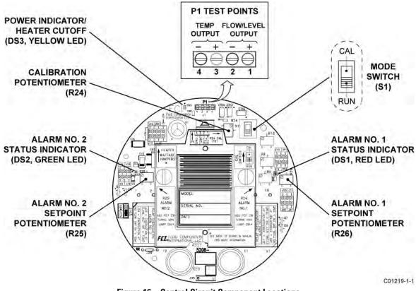
Figure 16 – Control Circuit Component Locations
