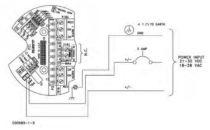
Figure 14 – 24 VAC/VDC Input Power Wiring Diagram
