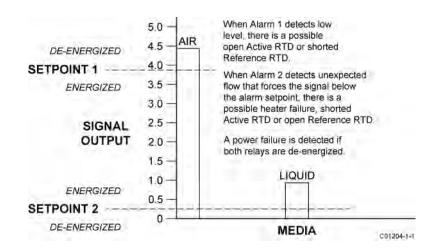
Figure 21 – Low Level Fail-Safe Alarm
