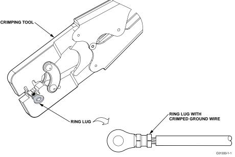
Figure 7 – Crimping Ground Wire Ring Lug
