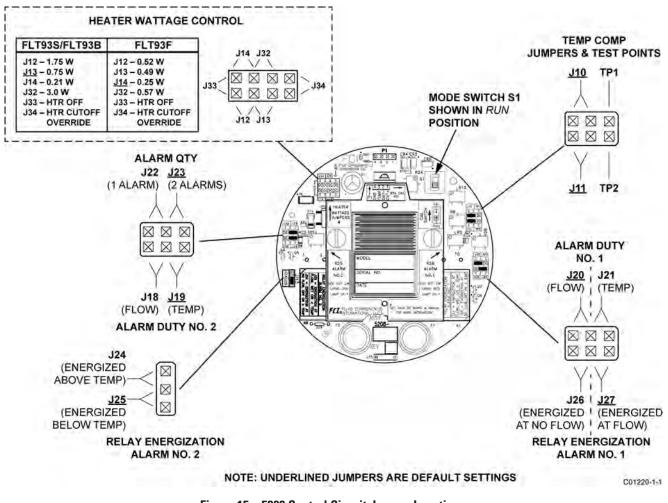
Figure 15 – 5208 Control Circuit Jumper Locations
