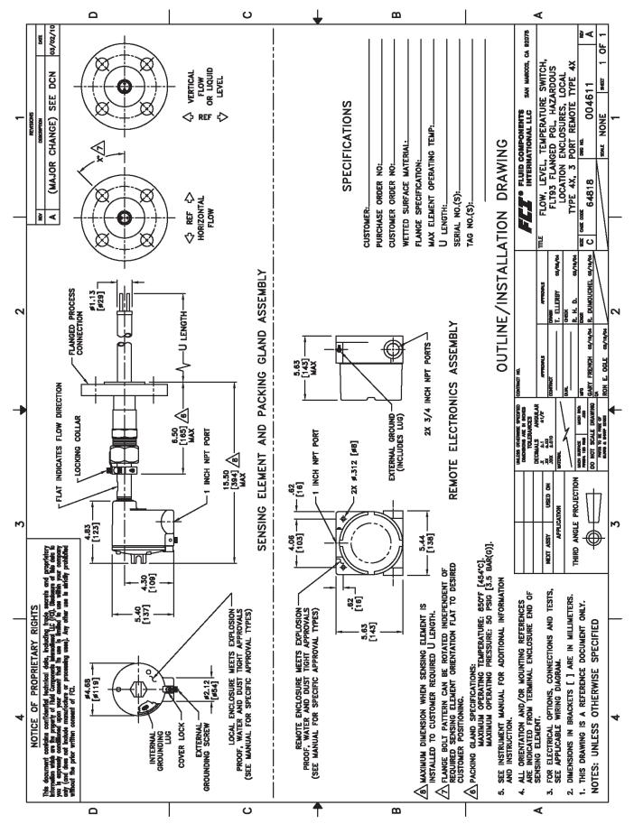
Flanged Low Pressure Packing Gland with Local Hazardous Location Type 4X Enclosure: 3-Port Remote Type 4X
