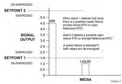
Figure 22 – High Level Fail-Safe Alarm
