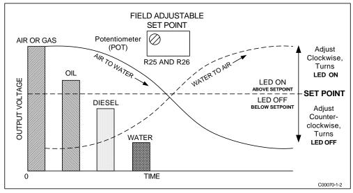
Figure 18 – Level Application Signal Output
