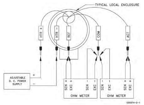
Figure 24 – Sensing Element Calibration Connections
