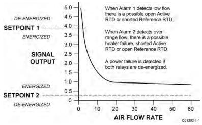
Figure 19 – Low Flow Fail-Safe Alarm
