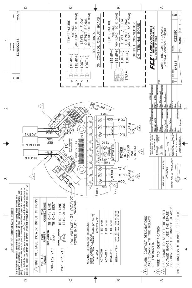
FLT93 Surface Mount: Local Wiring Diagram
