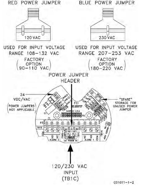
Figure 11 – Power Jumper Diagram
