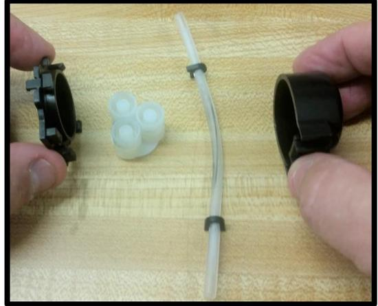
After clips are in place on the tube, wrap the tube around the roller assembly taking care that the clips line up with the slots in the front plastic housing. The opening in the clips faces outward when inserting into the pump head. Press them into place and then replace the back piece.
