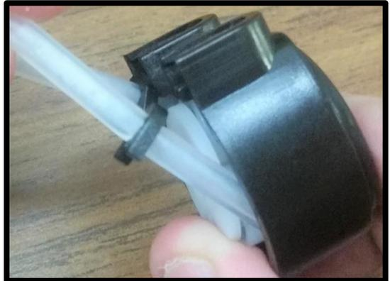
Once the pump tube is in place, put the pump head back onto the drive shaft and press in until the pinch points click into place so that the pump head is secure.
