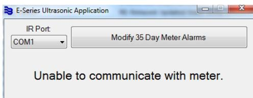
Make sure you have correctly installed the IR reader and selected the COM port to which it is connected.
