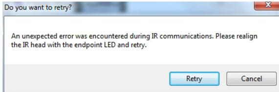
8. Realign the IR head and click **Retry**. If the retry fails, this message displays.
