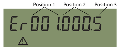
Figure 9: Alarm and operating mode screen in storage mode
