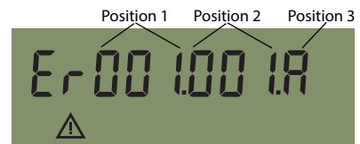
Figure 11: Alarm and operating mode screen in active mode
