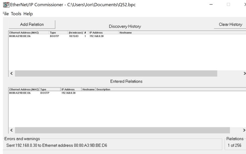
Figure 6 – Successful Detection of MAC ID and IP Address Assignment in BOOTP Server
