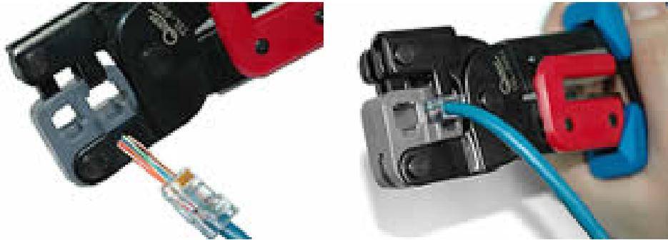
Figure 2 - RJ45 Crimp Tool
