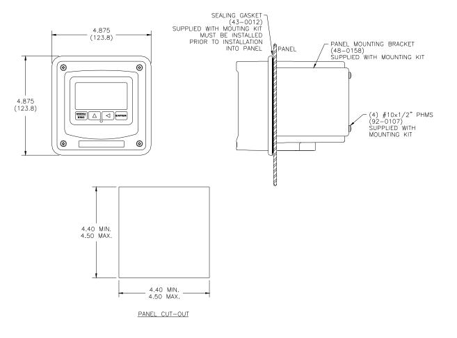
Figure 7 - Panel Mount Cut-Out
