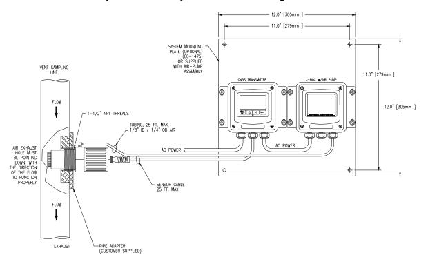
Figure 1 - Wet H2S Typical System Diagram
