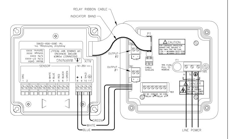
Figure 11 - Line Power Connection
