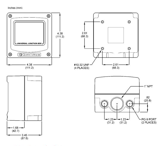
Figure 8 – Air Pump Enclosure Specifications
