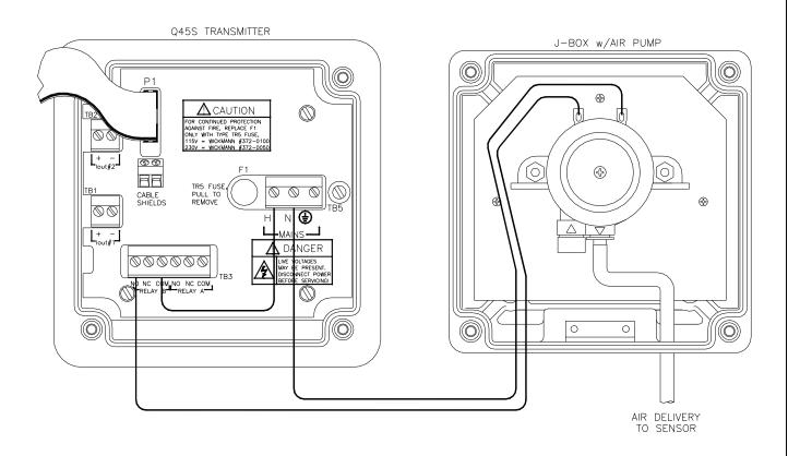
Figure 12 - Pump Interconnect Connection
