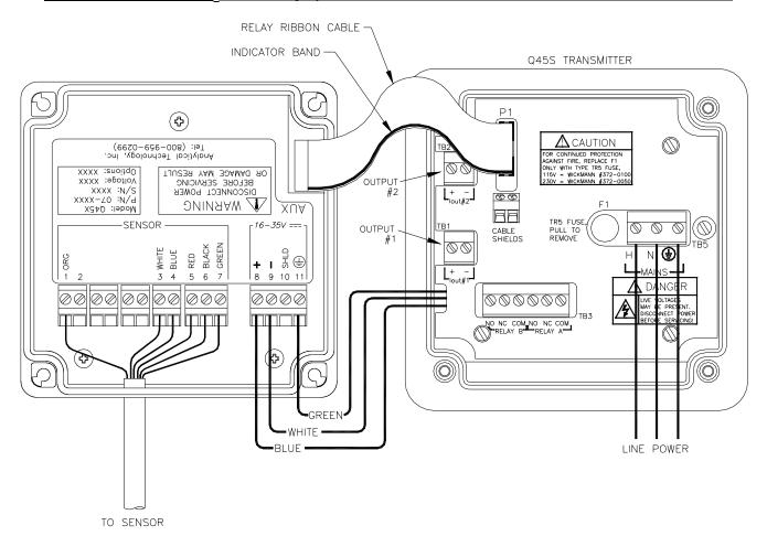
Figure 14 - Sensor Connection
