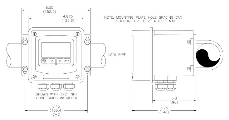
Figure 6 - Pipe Mounting Diagram
