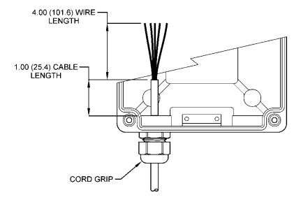
Figure 15 - Sensor Cable Preparation
