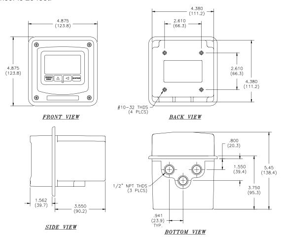
Figure 2 - Q45 Enclosure Dimensions, AC Power
