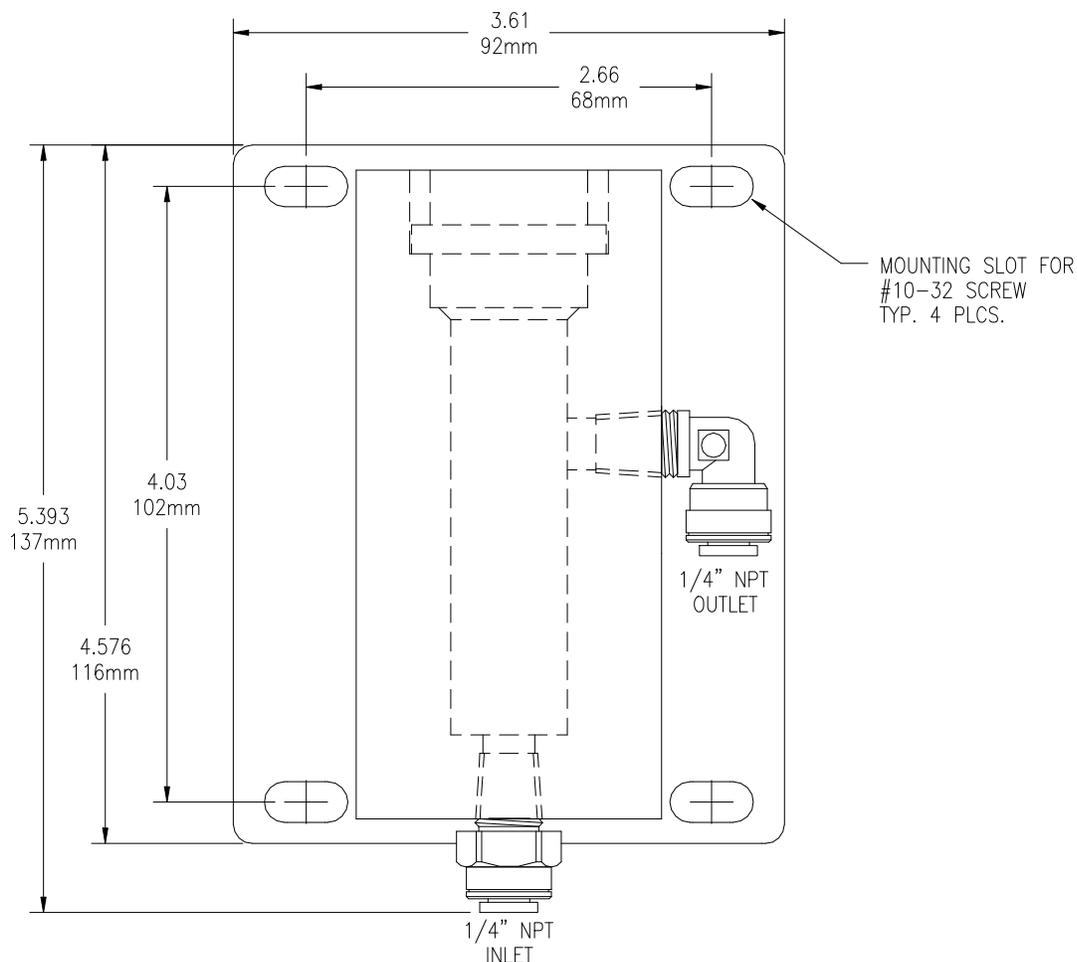
**Figure 16 - Sealed Flowcell Details**
