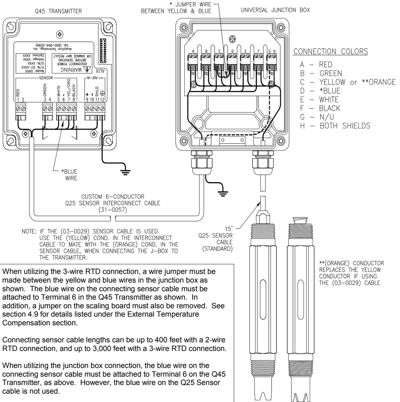
\* When utilizing the 3-wire RTD connection, a wire jumper must be made between the yellow and blue wires in the junction box as shown. The blue wire on the connecting sensor cable must be attached to Terminal 6 in the Q45 Transmitter as shown. In addition, a jumper on the scaling board must also be removed. See section 4.9 for details listed under the External Temperature Compensation section.
