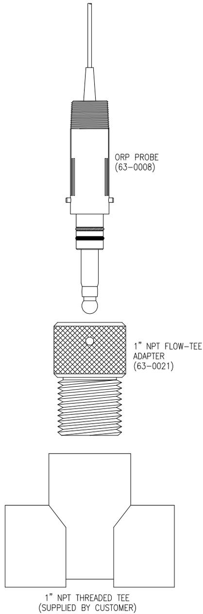
**Figure 17 - Twist-Lock Tee**
