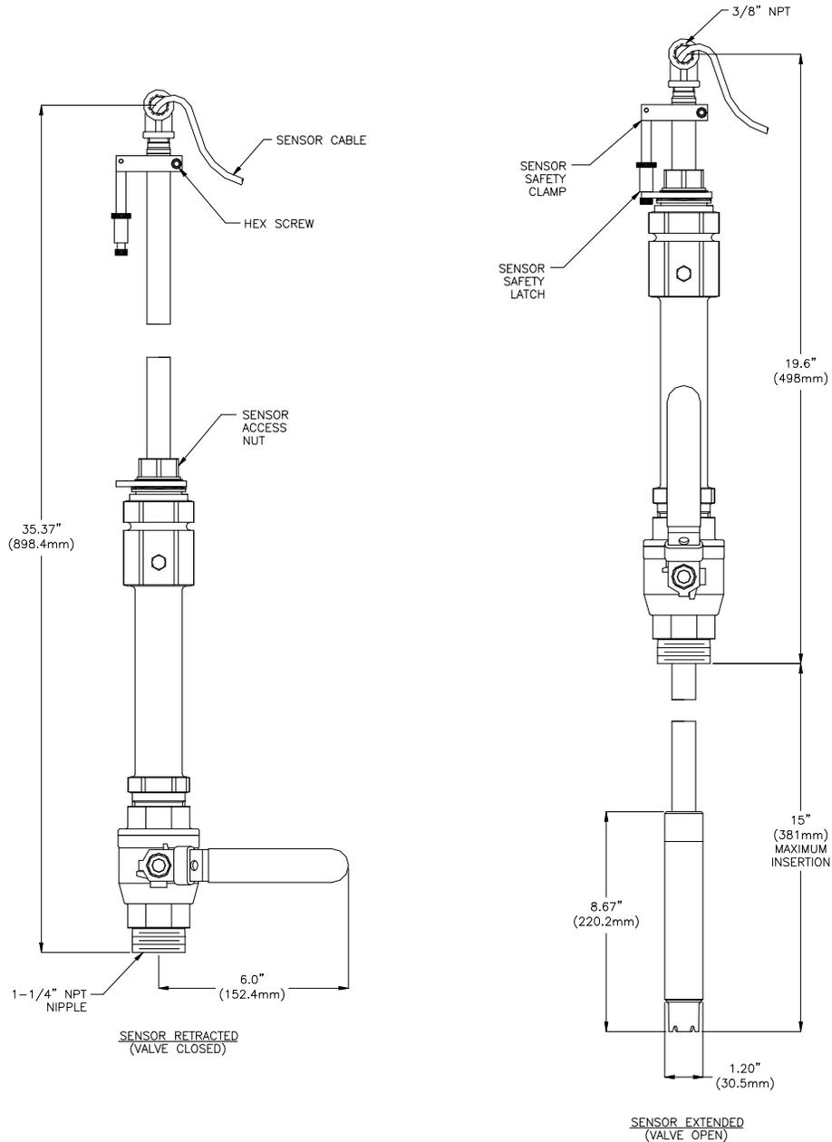
**Figure 12 - S.S. Sensor Insertion Mount**
