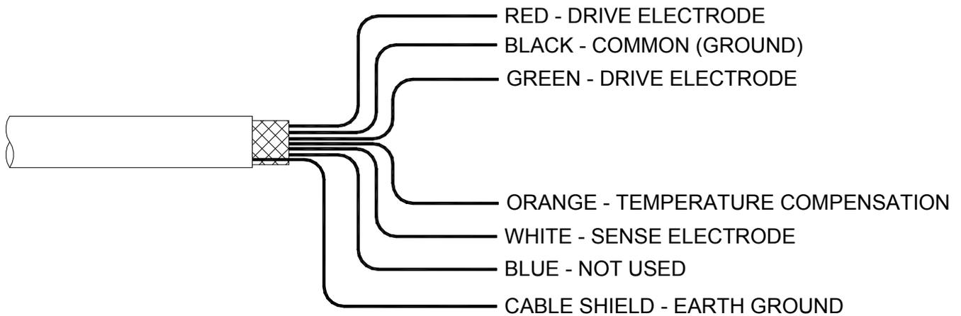
**Figure 24 - Detachable single Shielded Cable, Q25R**
