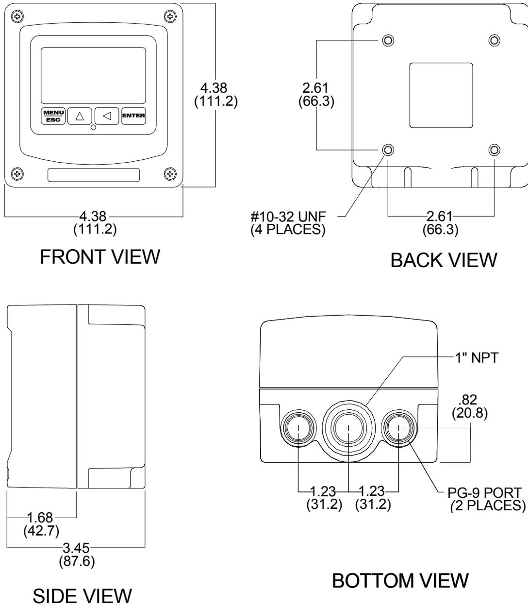
**Figure 2 - Q45 Enclosure Dim 2-Wire & Batt units**
