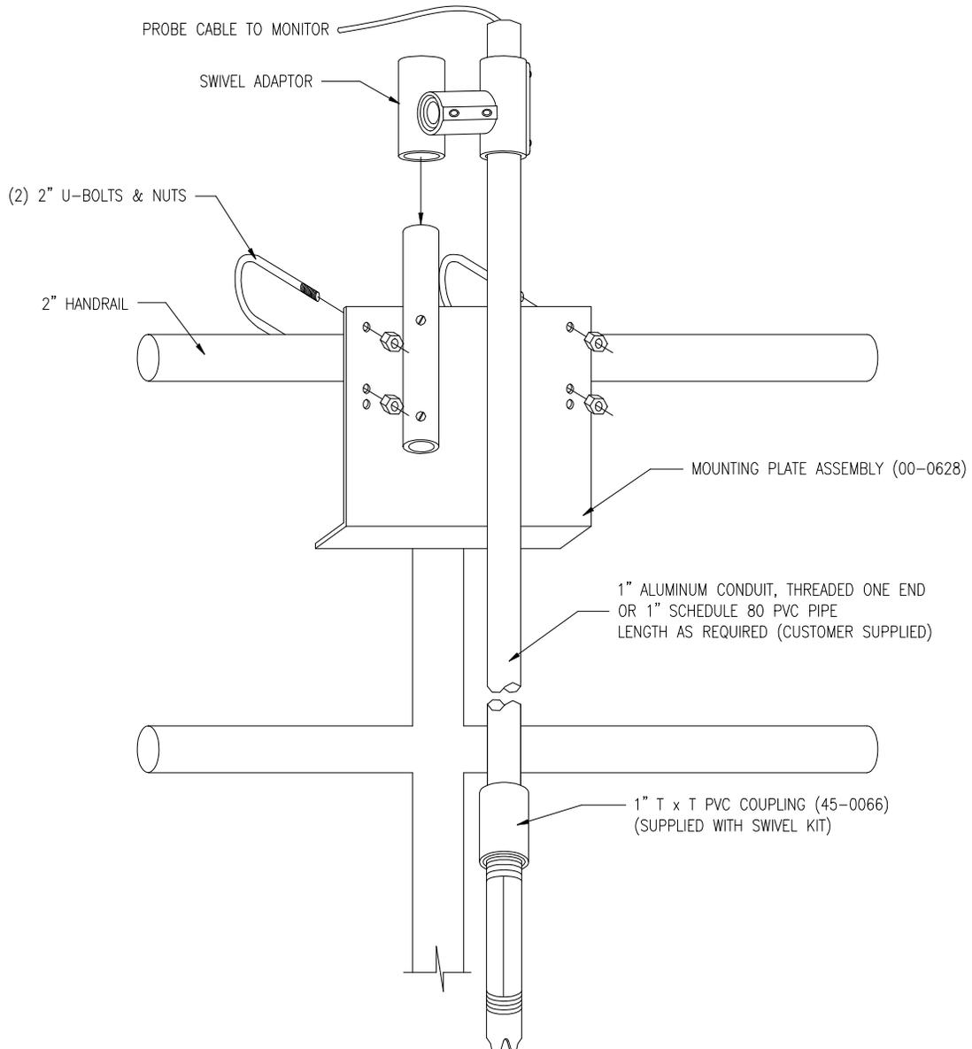
**Figure 11 - Sensor Submersion Mount**
