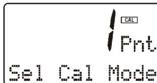
5. The system now begins acquiring data for the calibration value. As data is gathered, the units for ORP and temperature may flash. Flashing units indicate that this parameter is unstable. The calibration data point acquisition will stop only when the data remains stable for a pre-determined amount of time. This can be overridden by pressing ENTER. If the data remains unstable for 10 minutes, the calibration will fail and the message **Cal Unstable** will be displayed.
