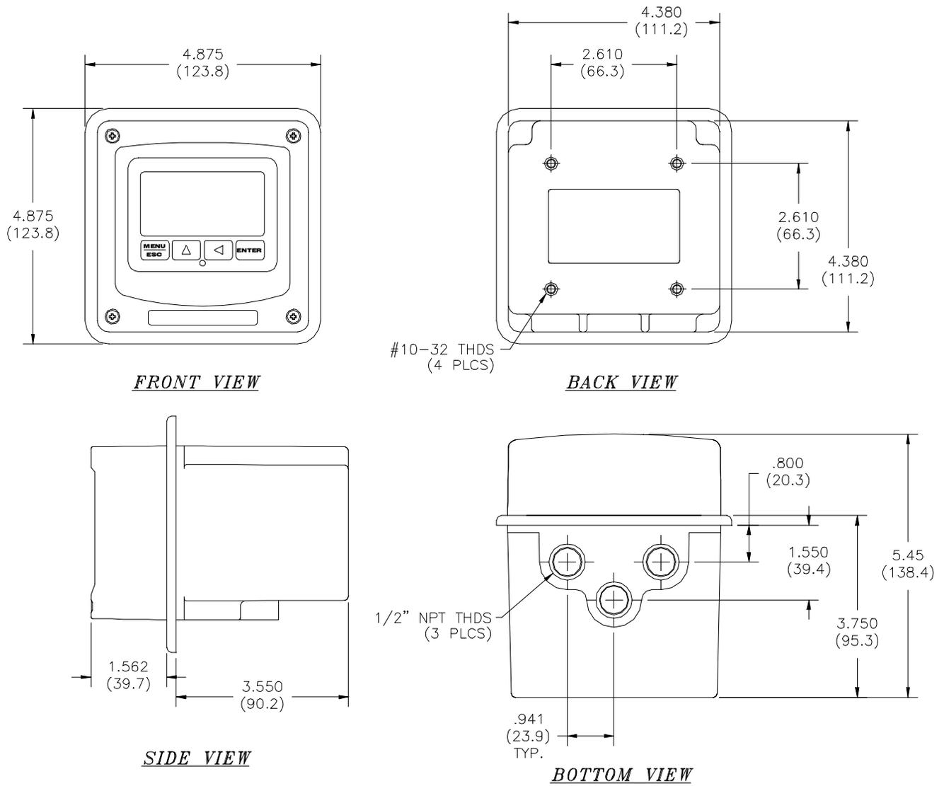
Figure 1 - Q45 Enclosure Dim AC Pwr units
