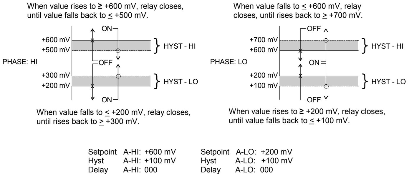
**Figure 33 - Alarm Relay Example**
