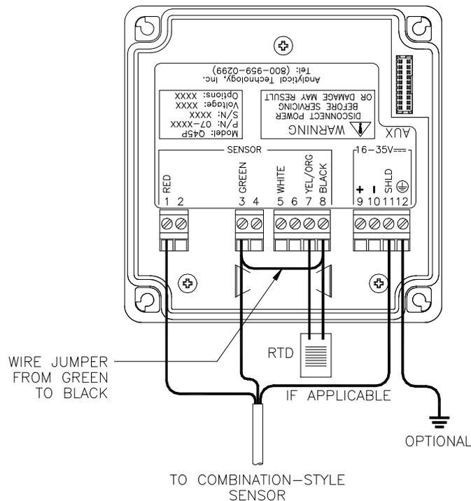
**Figure 27 - Sensor Connections, Combination Electrodes**
