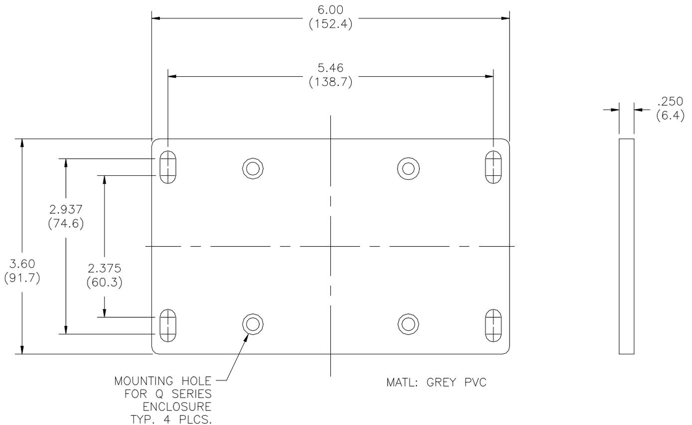
**Figure 3 - Wall or Pipe mount Bracket**
