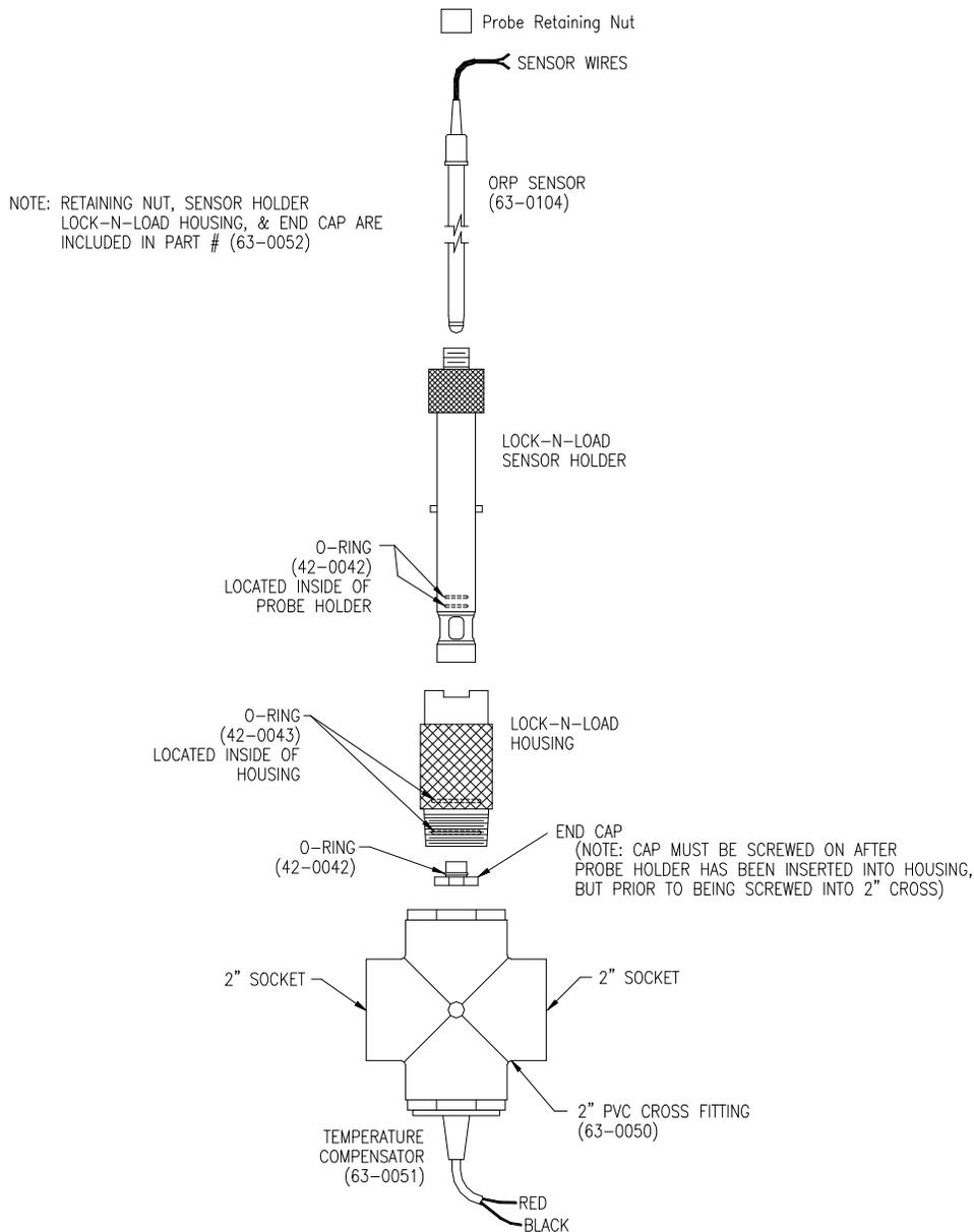
**Figure 18 - Lock-n-Load Sensor Exploded View**
