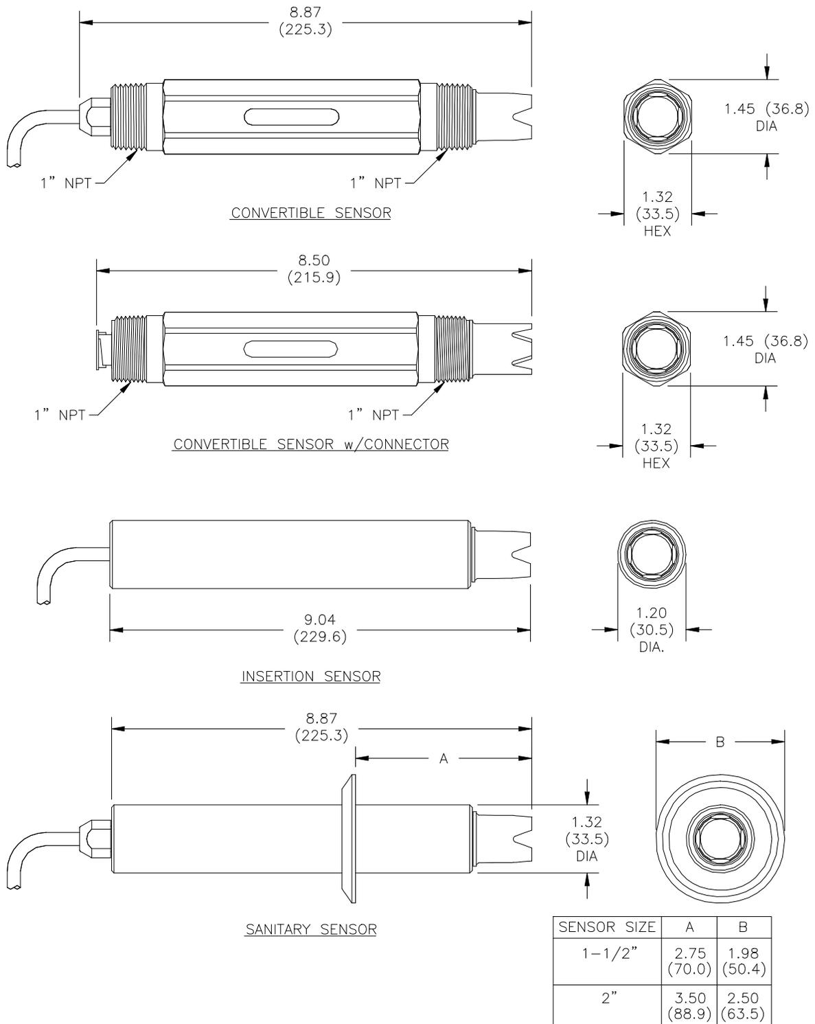
Figure 7 - Q25 Sensor Types
