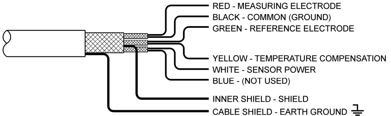
**Figure 23 - Cable Description, Model Q25**
