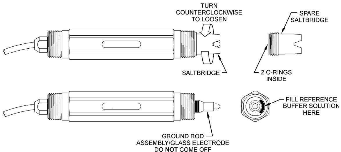
**Figure 35 - Replacing the Saltbridge and Reference Buffer**
