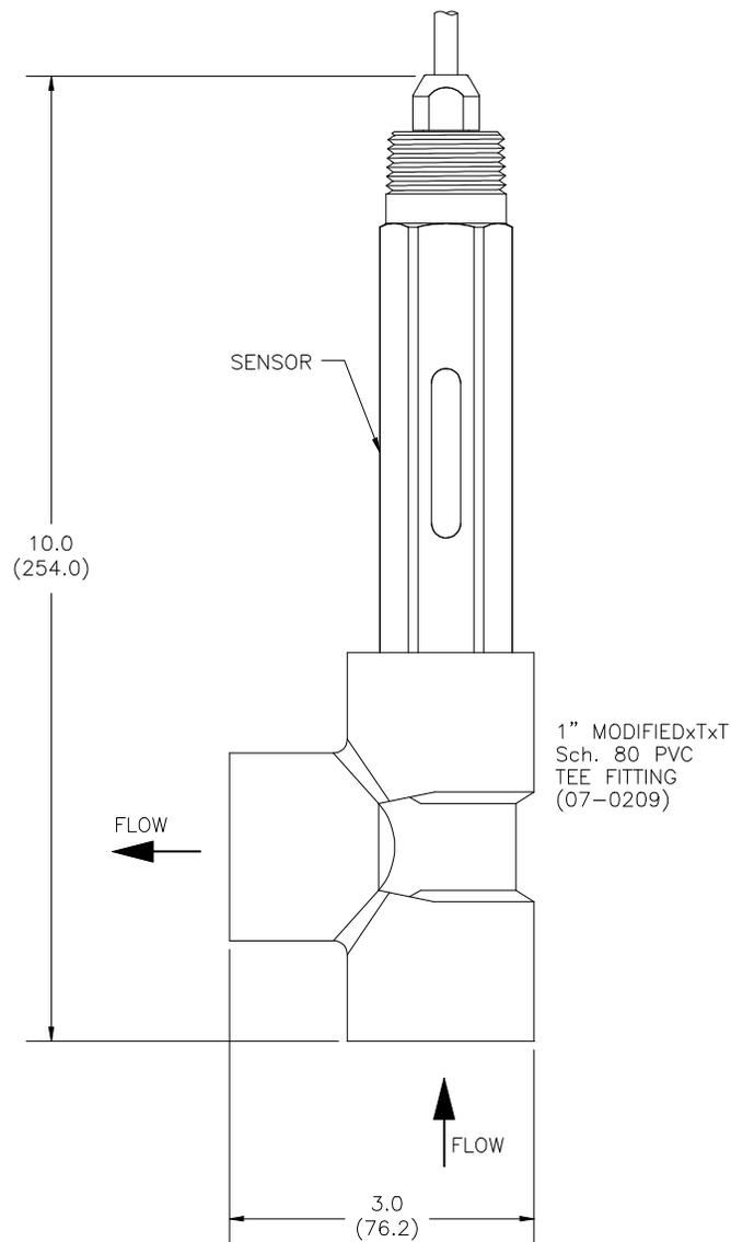
**Figure 8 - Flow Through Tee Mount**
