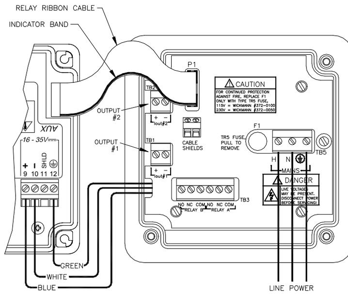
**Figure 20 - Line Power Connection**
