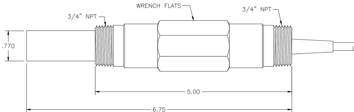
**Figure 15 - (63-0023) Combination ORP Sensor, Submersion**
