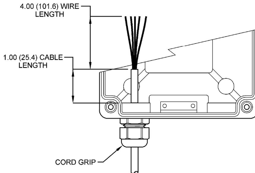
**Figure 25 - Sensor Cable Preparation**
