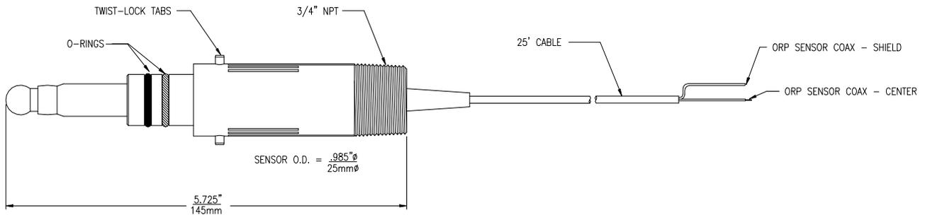
**Figure 14 - (63-0008) Comb. pH Sensor, Flow**
